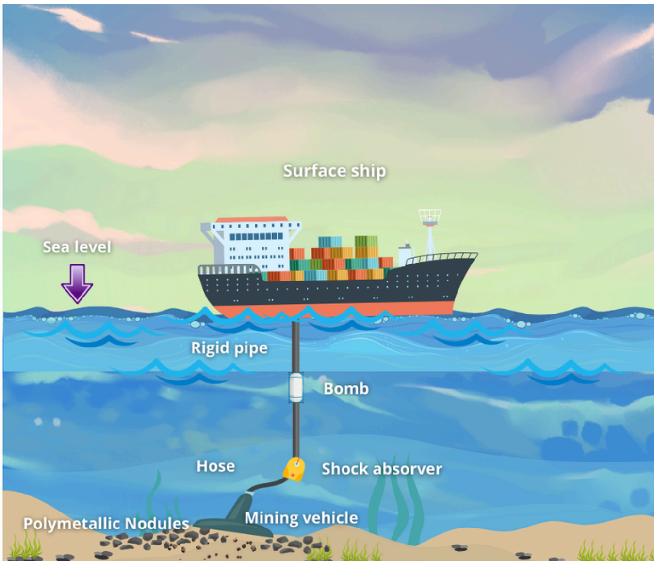
FIGURE 3. SCHEMATIC OF THE VERTICAL TRANSPORT SYSTEM (VTS) IN DEEP SEA MINING
